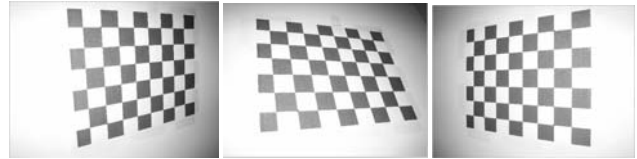
Fig. 6. Images for camera calibration from 3-planes, where each plane is located on separate images.
